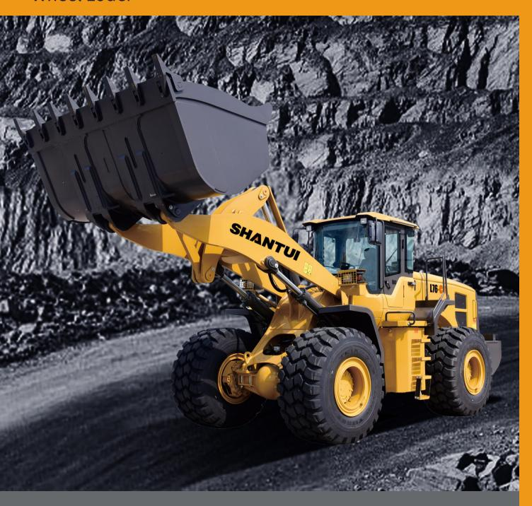
Engine WEICHAI WP10G286E301 Rated power 210kW Max. Breakout Force 185kN Operating weight 23680kg Bucket Capacity 4.5m³
