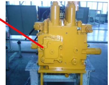
Main control valve
