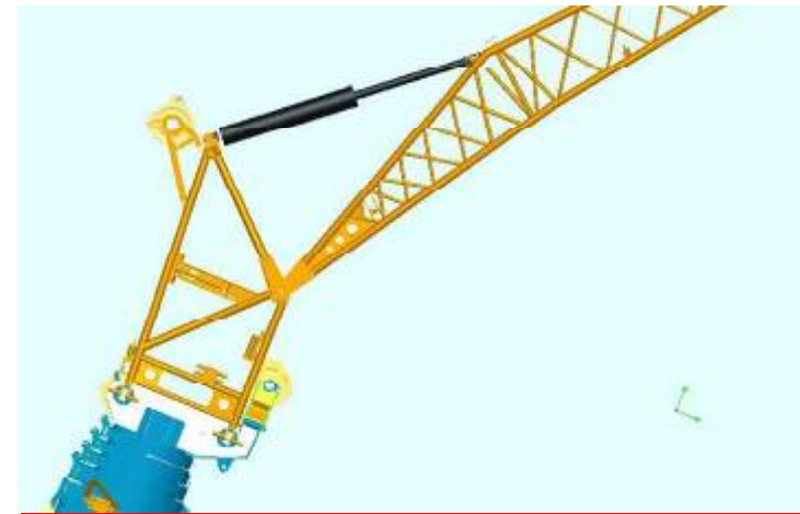
Automatic derricking Quick s continuous derricking within the range 0-40 degrees
